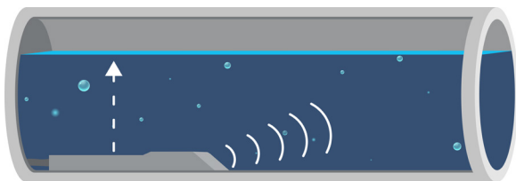
Submerged ultrasonic sensor measures level and velocity
