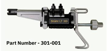
For use with the Staht Line Tester when testing safety lifelines with slip indicators fitted to the front end of termination (swage). The extension adaptor bypasses the slip indicator.
